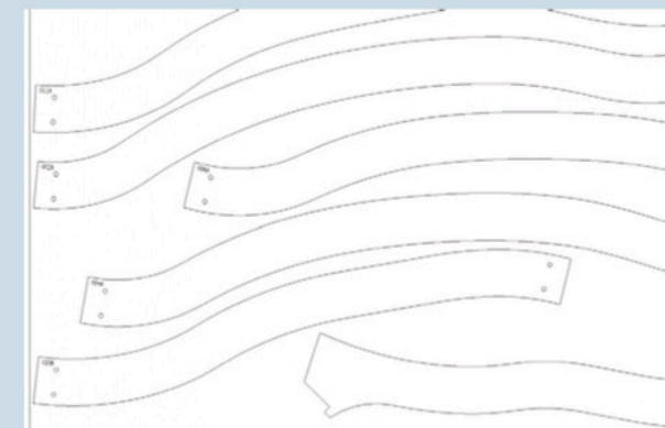
Figure 3: Result of one segment for CNC milling after nesting optimization
