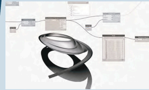
Figure 2: The Dynamo script used to translate the geometry to Revit
